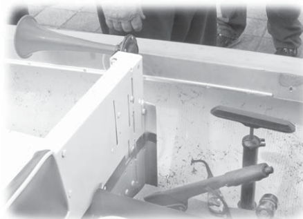
Nice details, like the air horn powered by a tire pump.
