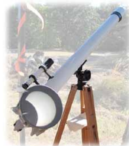
Solar projector made from funnel.
